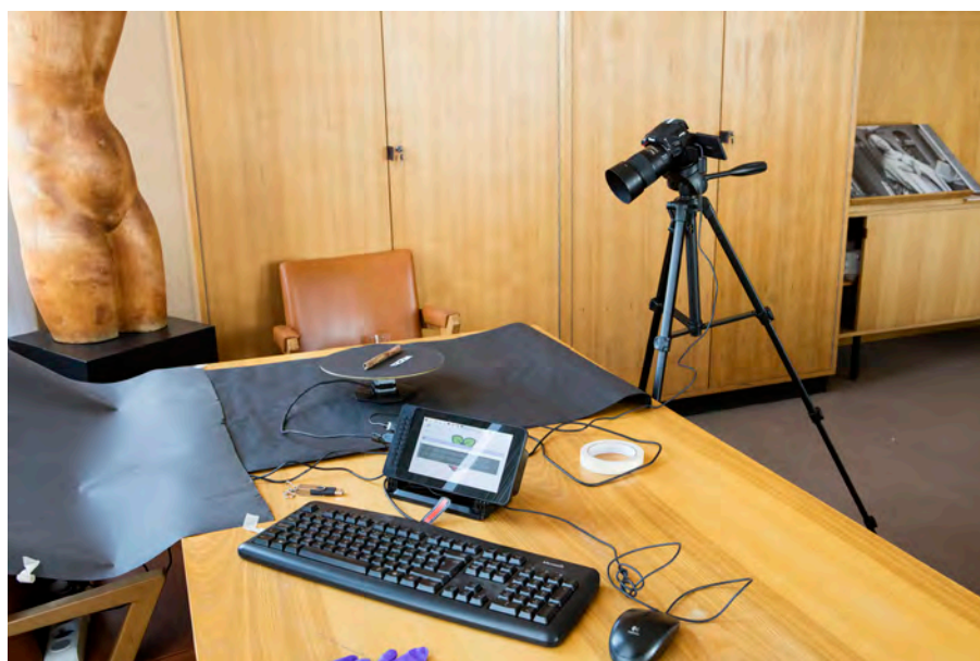
Fig. 5: Computerised turntable system with multi-camera setup developed at RLAHA accelerates the photographic documentation of relics for the creation of 3D photogrammetric images. Photo: G. Kazan
