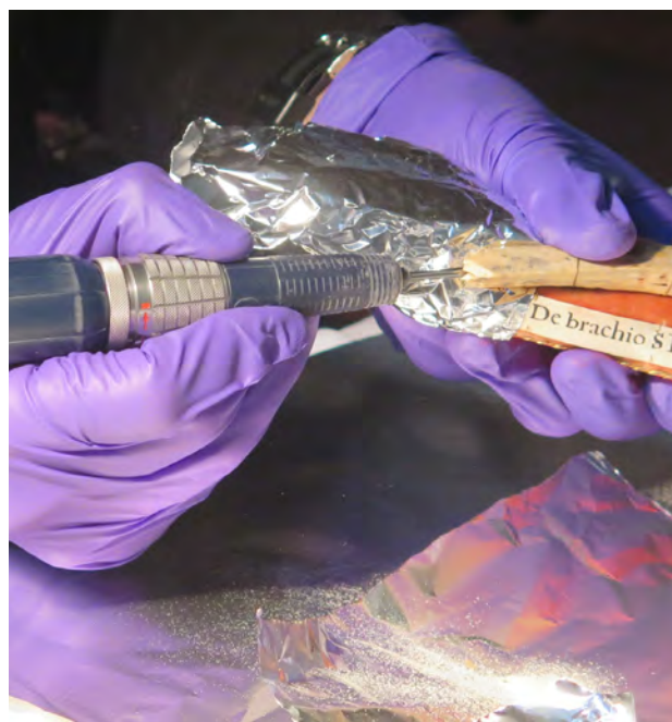
Fig. 8: A surgical drill is used to obtain bone powder from a relic using the “Keyhole” sampling method. The quantity of powder on the foil indicates the sample amount required for a successful radiocarbon date. Photo: Oxford Relics Cluster
